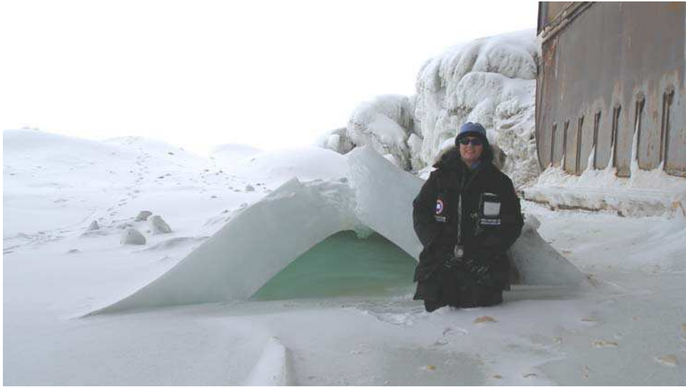
Fig. 2 Photograph showing ice buckling at the SDC in the Beaufort Sea (photo by the author)
