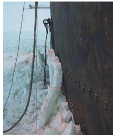
Figure 1: Large-scale ice bending on the SDC (Photo courtesy of S. McDermott)
