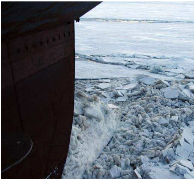
Fig. 3 Photograph of mixed mode failure including rubbing and splitting at the SDC in November 2005 (photo by the author).
