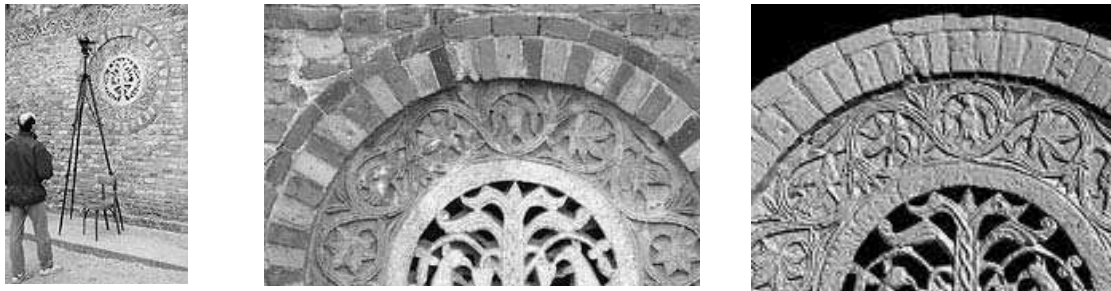
Figure 8: The Biris camera is shown mounted on a conventional tripod (left) scanning a rosone (middle) on the façade at the 8 th century Abbey of Pomposa near Ferrara, Italy. The archival digital model (right) records the surface shape and condition of the object after 1100 years exposure to the elements.
