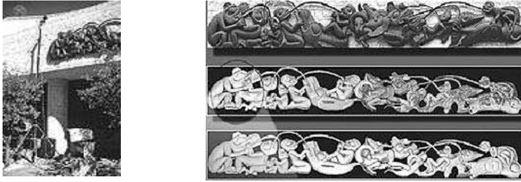
Figure 7: The Large Volume camera is shown on (left) mounted on a telescoping tripod to scan the sculpture Mythic Messengers at the Canadian Museum of Civilization. The sculpture, (top right), is mounted 4 m above ground on an exterior wall and measures 9 m long x 1.2 m wide. Over 100 scans were recorded as shown in the colour-coded image (mid right) and merged into a 3D model (lower right).
