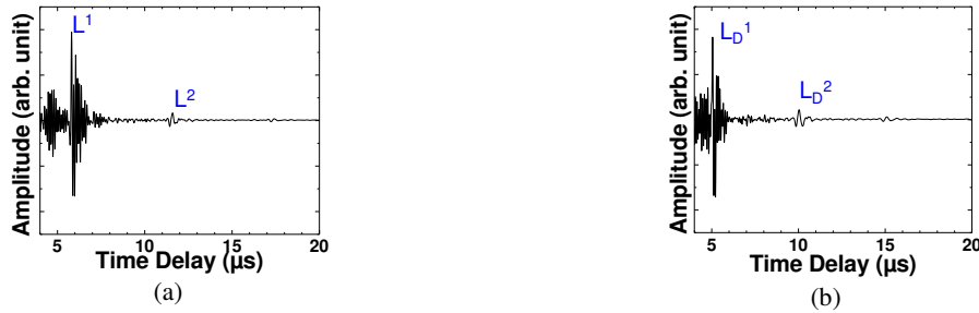
Fig. 9 Measured ultrasonic signals in time domain at room temperature at a location (a) without and (b) with disbond using the FUTs shown in Fig. 8.
