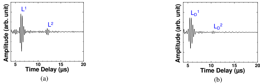
Fig. 11 Measured ultrasonic signals in time domain at room temperature at a location (a) without and (b) with disbond using the FUTs shown in Fig. 8 and an inductive non-contact method.
