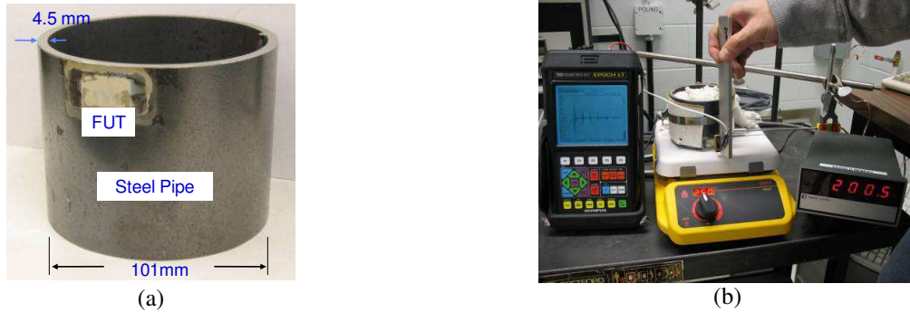
Fig. 2 (a) One FUT shown in Fig. 1 glued to a steel pipe with an O.D. of 101 mm and a thickness of 4.5 mm, (b) ultrasonic measurement at 200°C.
