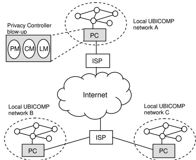
**Figure 4. Privacy-Preserving UBICOMP architecture (ISP = Internet Service Provider, small circles are UBICOMP devices, PC = Privacy Controller, PM = Policy Module, CM = Compliance Module, LM = Link Module).**
