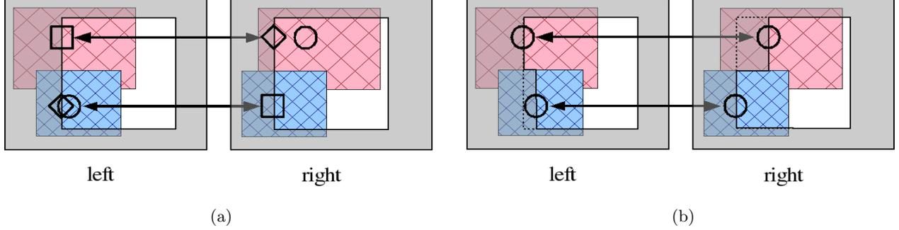
**Figure 3.** Stereo matching ambiguity along the boundary. (a) points along the boundary in one eye (square) can be matched in the other eye either to the boundary (diamond) or to the scene (circle); (b) the boundary is displaced so that it matches the underlying scene (circles).
