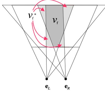
**Figure 4.** Viewing geometry. The fovea frustum is contained within the frustum of the peripheral image. Only points in the  $\mathcal{V}_f$  area can be perceived in stereo at high resolution; points in  $\mathcal{V}_f^*$  are visible only in one of the two fovea images.
