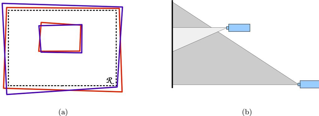
**Figure 2.** Projection geometry: (a) the footprints of the four projectors need only be roughly aligned, with overlap between left and right images in both periphery and fovea; (b) fovea projectors must not create shadow in the light path of the periphery projectors.
