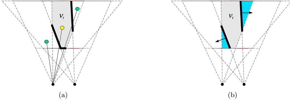
**Figure 5.** Testing whether a point lies inside or outside  $\mathcal{V}_f$  in the left eye images: (a) stencil-based inclusion test; (b) depth buffer method to remove points *outside*  $\mathcal{V}_f$  in the periphery image.
