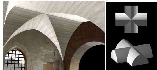
Figure 8: Left: Groin vaulted ceiling modeled with 3ds max ® . Right: Two arches extruded at right angles form a mould for the ceiling model.
