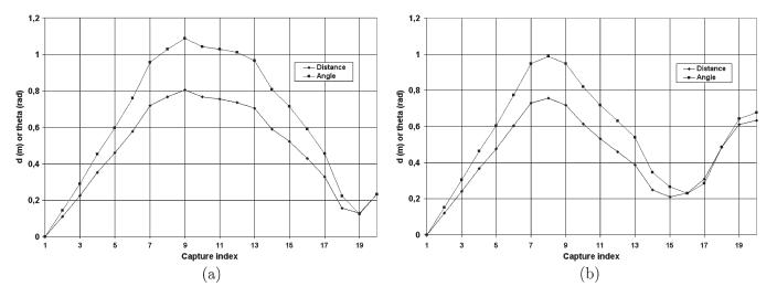
Fig. 4. (a) Angle and distance of the left camera with respect to the first capture. (b) Angle and distance of the right camera with respect to the first capture.
