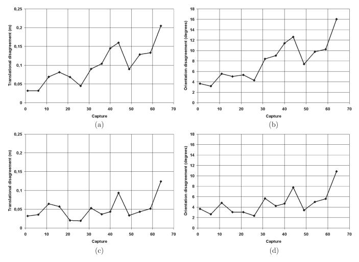
Fig. 8. (a) Position disagreement between bundle adjustment and the proposed method without error correction. (b) z-axis orientation disagreement between bundle adjustment and the proposed method after error correction. (c) Position disagreement between bundle adjustment and the proposed method after error correction. (d) z-axis orientation disagreement between bundle adjustment and the proposed method after error correction.
