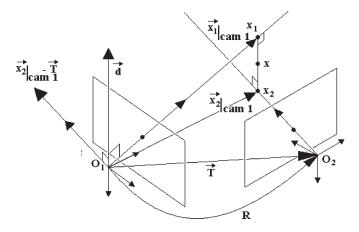
Fig. 2. Geometry of the triangulation procedure.
