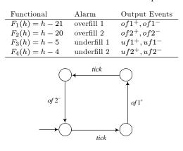
Fig. 3. The tank controller specification.
