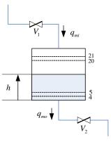
Fig. 2. Tank control schematic,  $V_1$  and  $V_2$  are control valves.
