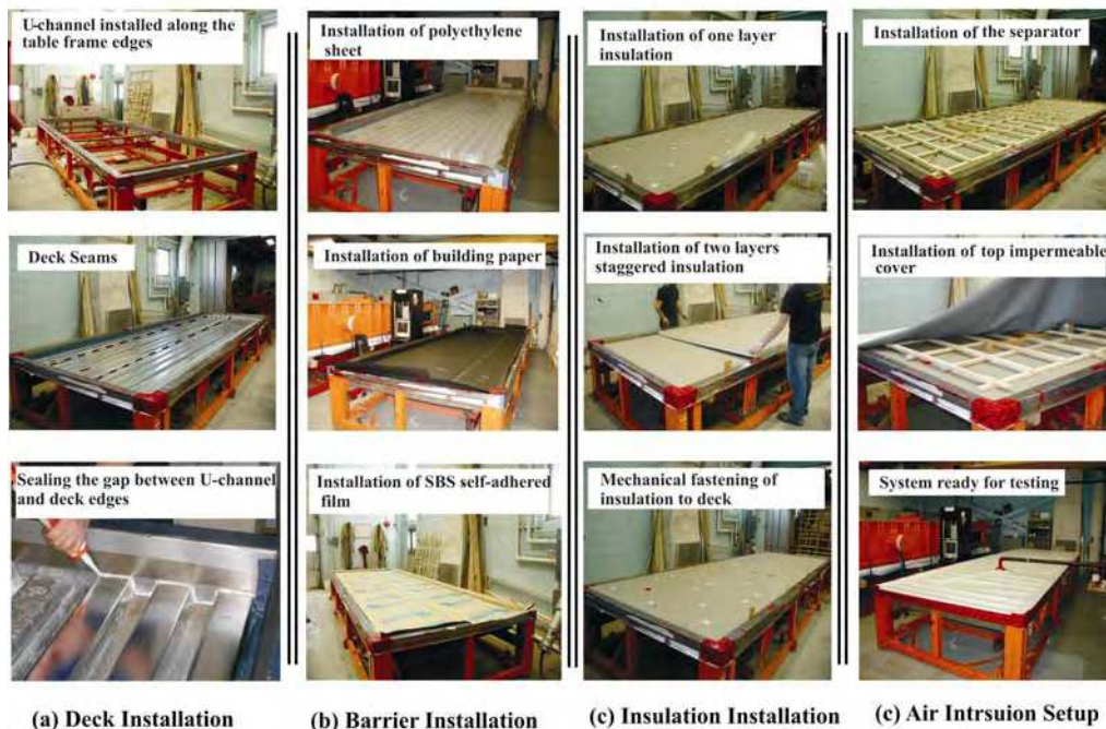
Figure 3: Experimental set up of the test assemblies
