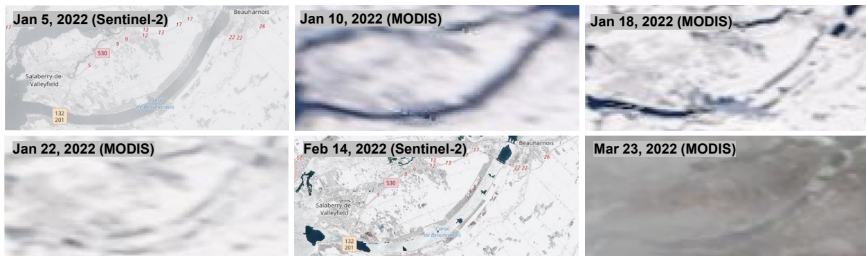
Figure 4. Optical images of Beauharnois Canal used for labelling of pixels as ice or water.
