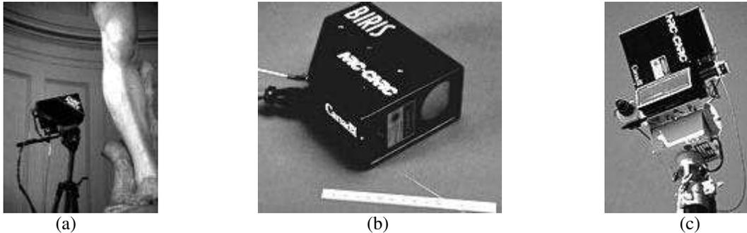
**Figure 1.** The High Resolution Laser Scanner (a), shown imaging the right leg of Michelangelo's *David*, can be mounted on a tripod for high resolution monochrome imaging of details such as tool marks. The Biris 3D Laser Camera (b) can be mounted on either a conventional tripod or on a linear translation stage for scanning. The Large Field of View Laser Scanner (c) can be mounted on a telescoping tripod and raised to a height of 10 m to scan large objects such as outdoor sculpture.
