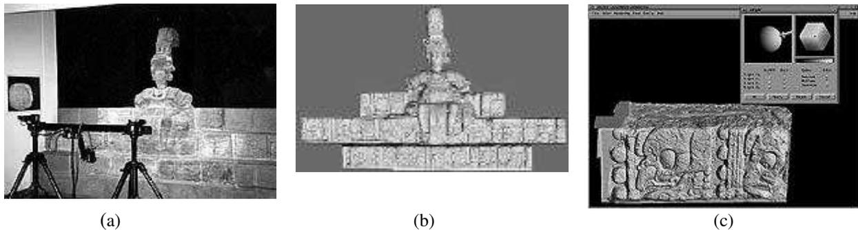
**Figure 3.** The Biris camera mounted on a linear translation stage (a) was used to scan the 3.4 m wide x 2.3 m high Hieroglyphic Stairway at the Peabody Museum in Boston to produce a 3D digital model (b). The software also enables the data to be used for research applications. Similar to the use of raking light to examine details on works of art, researchers can interactively move the light source to any angle and zoom in to examine features such as details on the steps (c).
