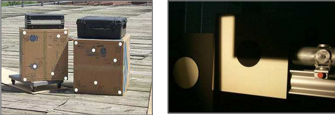
Figure 11: Demonstration under direct sunlight illumination and analysis of worst case scenarios of on-orbits light conditions by removing the optical interference filter inside the laser scanner head.
