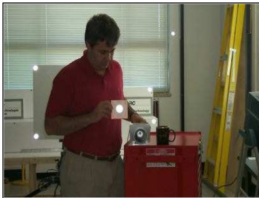
Figure 10: Demonstration of lighting robustness of the laser scanner under direct illumination. The video camera was moved in order to be able to take this picture and the light source is directed exactly toward the laser scanner.
