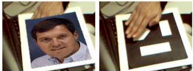
Figure 7 – Successful augmentation onto a partially occluded pattern
