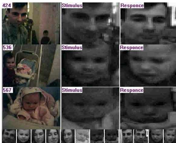
Figure 8: Recognizing users of the system out of 4 memorized: a frame grabbed (left column), a face extracted (middle column), a the association retrieved (third column).
