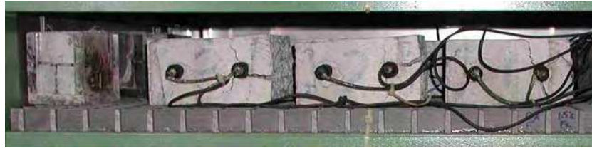
Corroding CS (1.5 wt% Cl - ) coupled with passive CS (0% Cl - )
