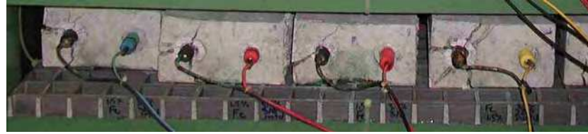
Corroding CS (1.5 wt% Cl - ) coupled with SS (3.5 wt% Cl - )
