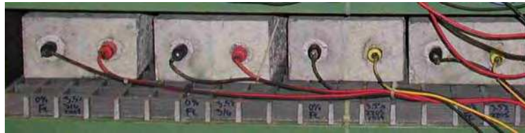
Figure 10. Photos of concrete specimens in which the passive CS (in concrete with 0% \text{Cl}^- ) was coupled with different types of SS (in concrete with 3.5 wt% chloride ions). No cracks can be observed in the concrete specimens.
