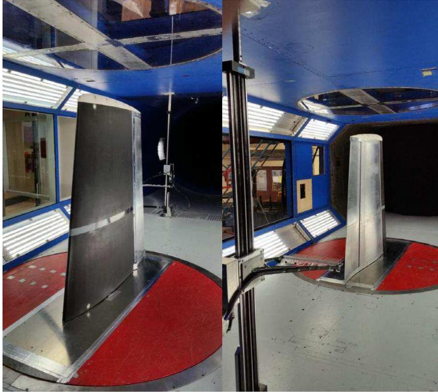
**Figure 7 MDO 505 wing model setup in the wind tunnel test section**
