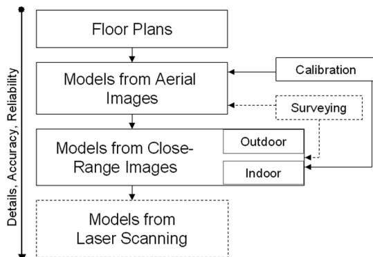
Figure 3: Hierarchy of model assembly (dotted means optional).
