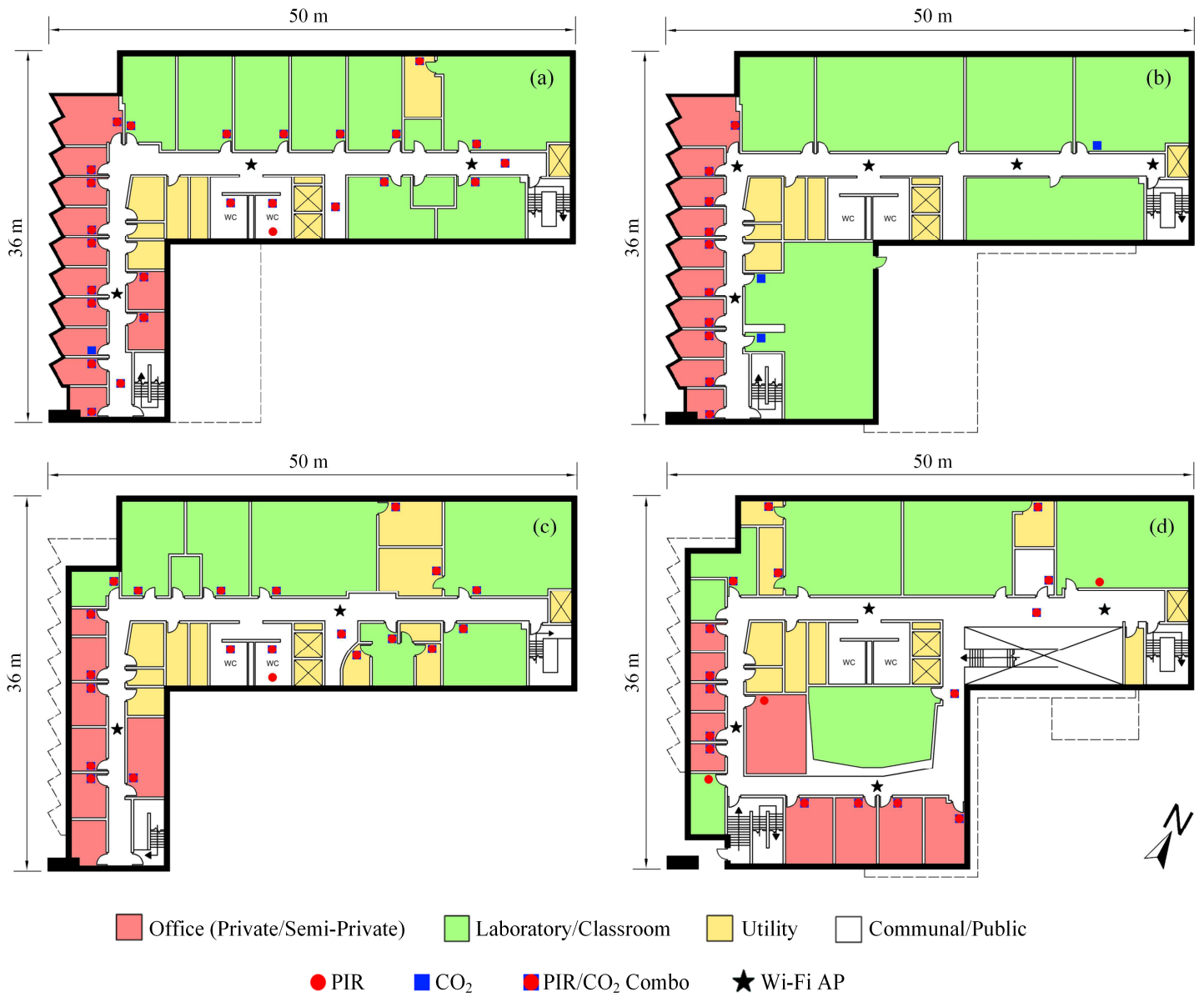
Figure 1: Floor and sensor configuration for (a) floor A, (b) floor B, (c) floor C, and (d) floor D.
