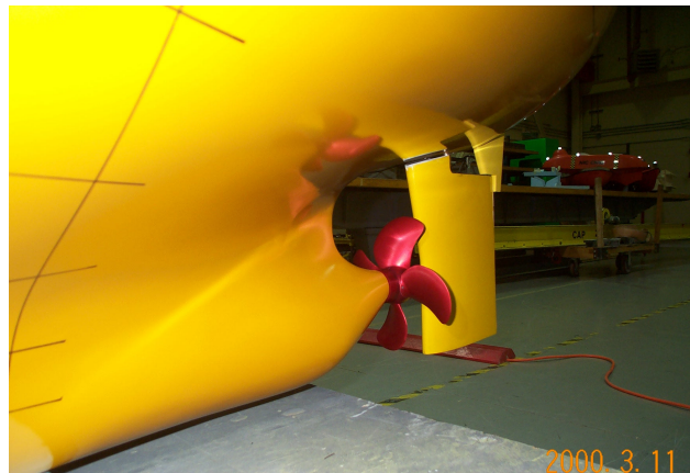
Figure 7, Single screw stern arrangement; Suezmax sized tanker designed for operation in light ice
