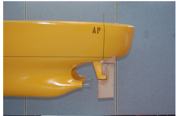
Figure 2, Twin gondola stern for Aframax sized tanker designed for moderate to heavy ice.
