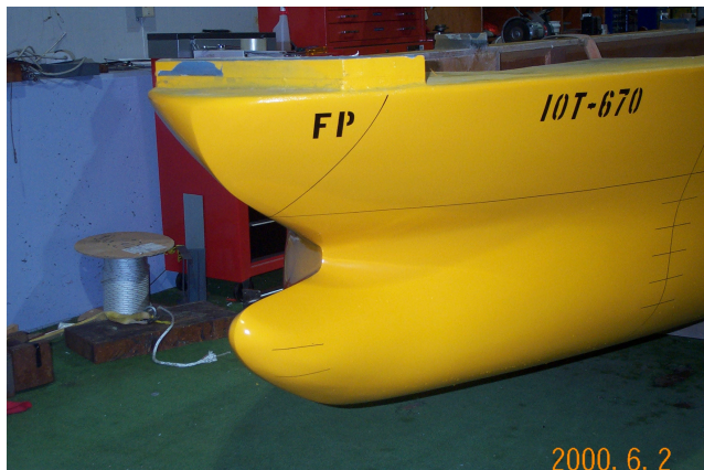
Figure 8, Modified bulbous bow for ice, Suezmax sized tanker designed for operation in light ice
