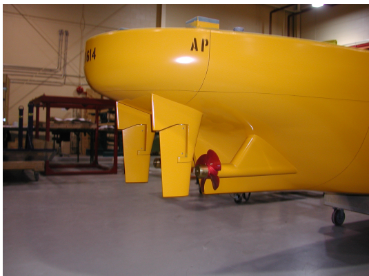
Figure 3, Twin propeller shafts and rudders, Suezmax sized tanker designed for moderate to heavy ice
