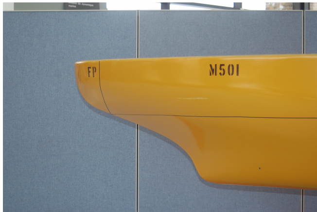
Figure 1, R-class style bow for Aframax sized tanker designed for moderate to heavy ice.
