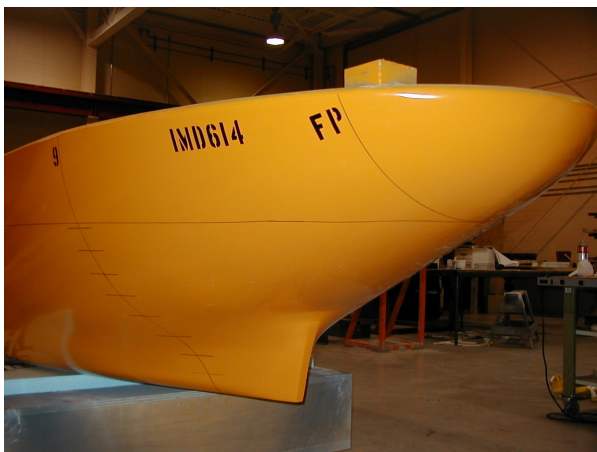
Figure 4, Spoon bow, Suezmax sized tanker designed for moderate to heavy ice
