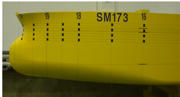
Figure 6, Bulbous bow for conventional tanker
