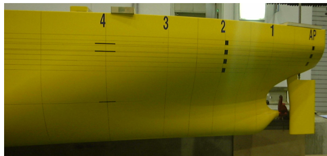
Figure 5, Stern arrangement for conventional tanker
