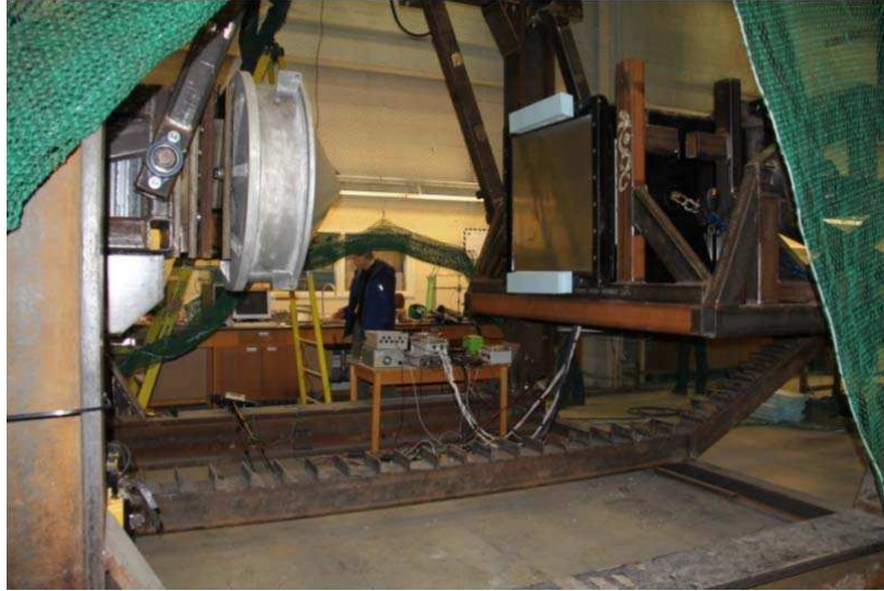
Figure 2. Photograph showing a partial view of the double-pendulum impact apparatus with the ice holder pendulum (left) and Impact Module pendulum (right) in the raised position for a test. The ‘toothed’ rail structure directly below the pendulums is the catch mechanism as shown in Figure 1. Protective netting is visible at the sides and in the background of the image. An overhead crane is used for lifting the pendulum masses to the desired elevation for a test.
