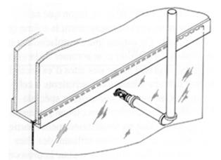
Figure 1 Sprinkler located at top of glazing
