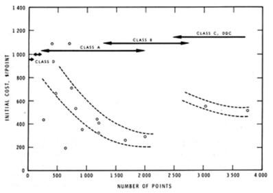
Figure 2. Correlation between the number of points and the initial cost/point of CCMS.
