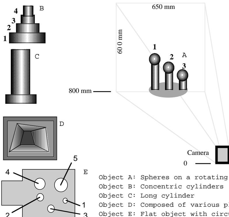
Figure 5: Camera set up for evaluation tests and test objects. better than 0.005 mm. The precision reported in fig. 3 are well above that value, thus, the CMM measurements are within the standards. Because of the limited number of pages, most of the results are given for the **RAL** scanner. For this scanner, the field of view (FOV) used for the reported tests is about 650 mm by 600 mm when the objects are placed at about 800 mm from the camera.
