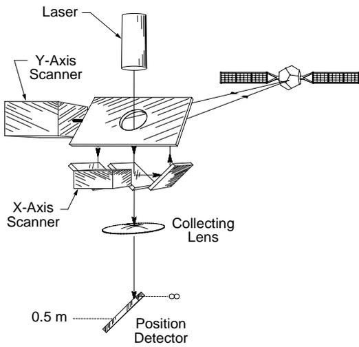
Figure 1: Auto-synchronized scanner.
