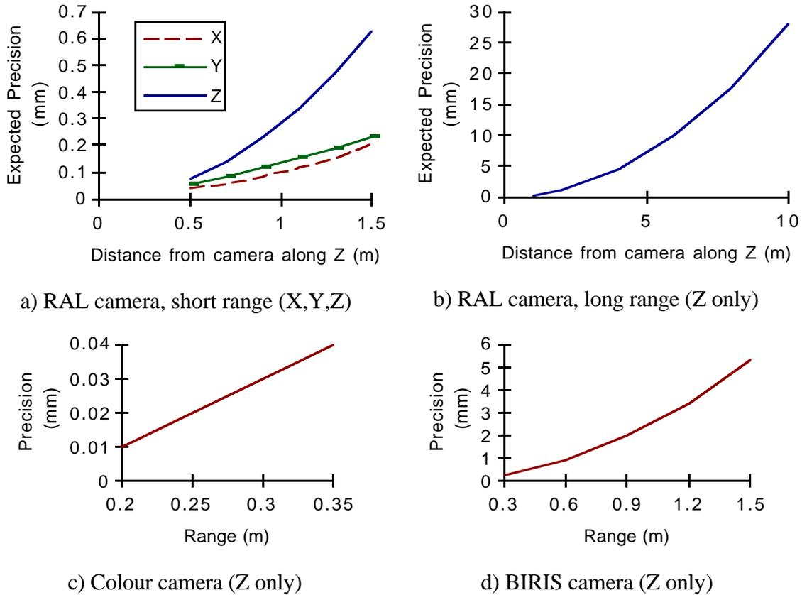
Figure 3: Expected precision of the range cameras.
