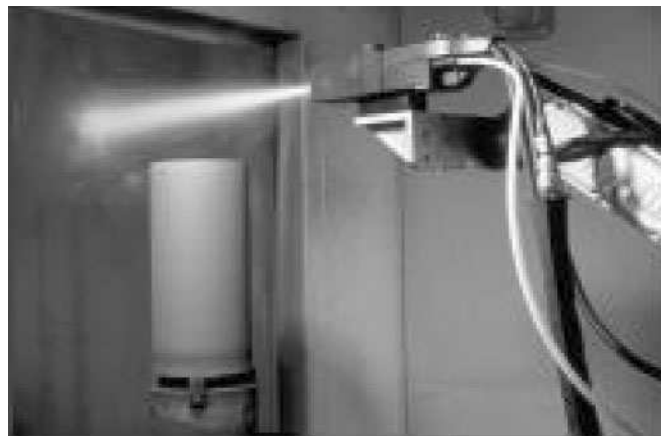
Fig. 1. A typical arc spray process in operation - JP 9000 system shown.
