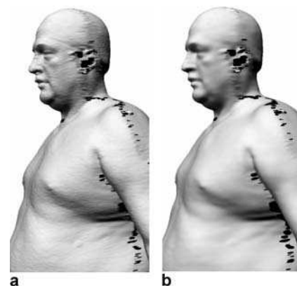
Fig. 2a,b. Surface smoothing of a 3D human scan using Taubin filter. a Original model. b Filtered model: the distribution of the displacement between the original and the filtered model is characterized by a mean value of 0.4 mm and a standard deviation of 0.52 mm
