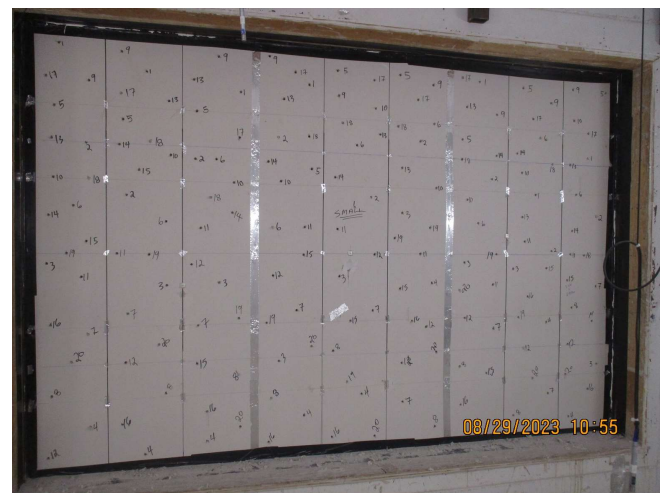
Figure 7: Image of the wall with twenty holes per bay (Case 12), resulting in one hundred and twenty holes in the wall.
