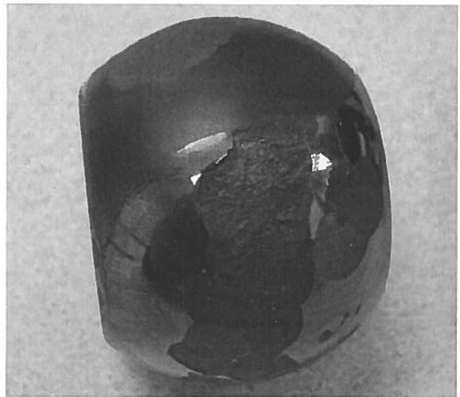
Figure 1: HVOF \text{Cr}_3\text{C}_2 -NiCr coating exhibiting cohesive failure after 1 year in service.
