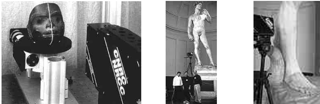
Figure 1. The High Resolution Color Laser Scanner (left) imaging the Tsimshian Stone Mask from the Canadian Museum of Civilization. In this configuration, the scan is made by rotating the mask 360° on a rotation table. The scanning mechanism projects a white laser spot (white line profile) on the mask from a RGB laser. The Scanner mounted on a tripod (center) is used in monochrome mode operation (red laser spot) to scan tool mark details on the leg of Michelangelo's David (right).
