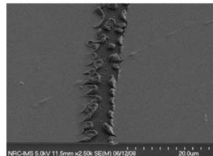
Figure 4. Chromium and amorphous silicon layer ablated by laser
