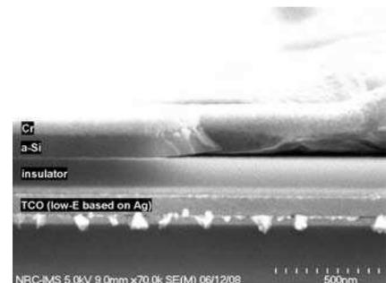
Figure 5. SEM cross-sectional view pointing out that the ablation only affected the Cr and a:Si layers
