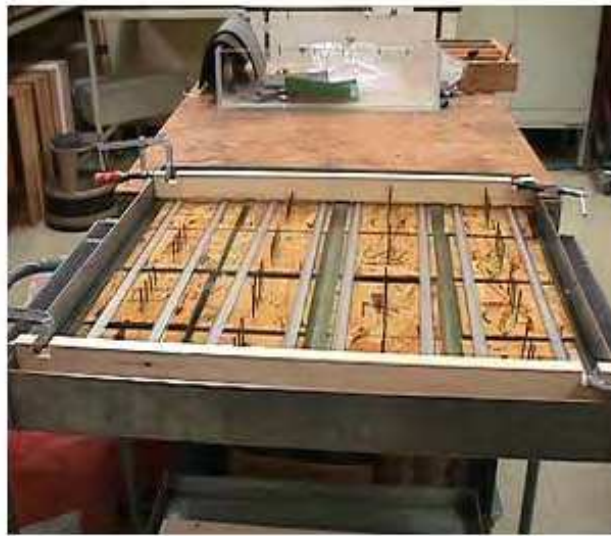
FIG. 3—Pre-conditioning of OSB Samples
