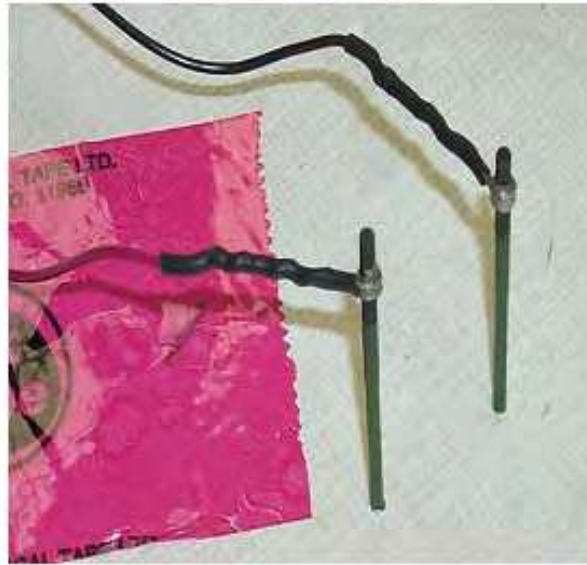
FIG. 2—Moisture pins inserted in OSB sample
