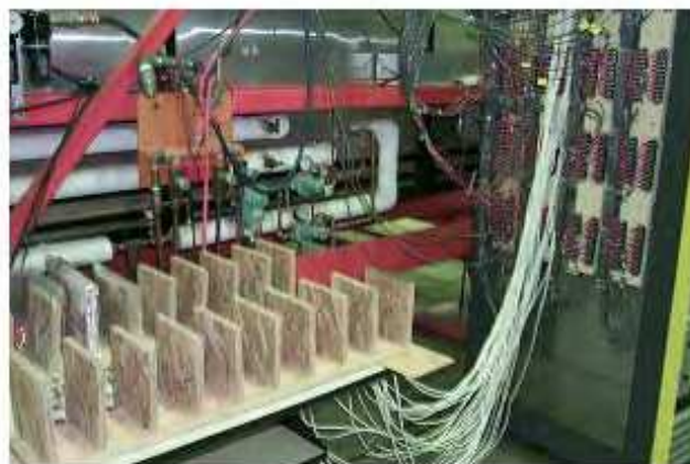
FIG. 5—Calibration of the moisture pins on OSB
