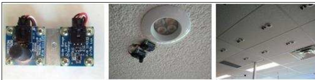
Figure 3. The sensor groups, their location next to the LED luminaires and overall layout on the ceiling.
