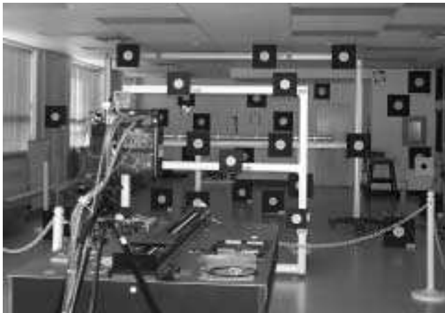
Figure 9: Tracking structure used for pose evaluation. Three groups of targets at different ranges are used to evaluate the performances and stability of the photo-solution.
