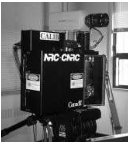
Figure 2: Prototype of the laser scanner system. A conventional video camera is “temporarily” mounted on the laser scanner for monitoring and comparison with conventional methods. Dimensions are 27 cm \times 18 cm \times 10 cm..
