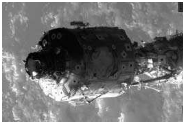
Figure 1: Example of the effect of sun illumination and earth albedo on video images. The Space Vision System [1,6] uses the known location of the B/W targets to compute the pose of the object(s). Even if this picture is of excellent quality, high contrast between illuminated and dark regions, and shadows are very problematic for automated space vision.
