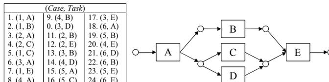
**Fig. 1.** Example log and corresponding workflow diagram.
