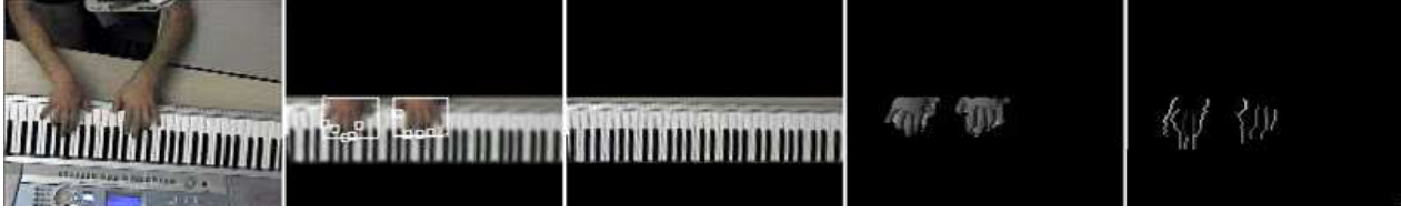
Figure 3. The stages of pianist hand and finger detection: 1) keyboard image rectification, 2) hand tracking, 3) finger location estimation.
