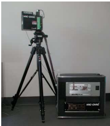
Figure 2: 3D laser scanner on a rigid tripod for field utilization. The quality of the tripod can provide relative stability. However, vibrations and oscillations induced by wind, people, or passing vehicles can seriously degrade the accuracy of the system.
