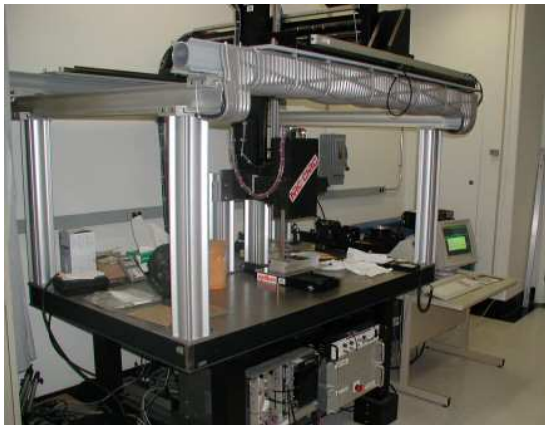
Figure 1: Lab configuration, rigidity between the scanner and the object is obtained by the use of a stable mechanical infrastructure.
