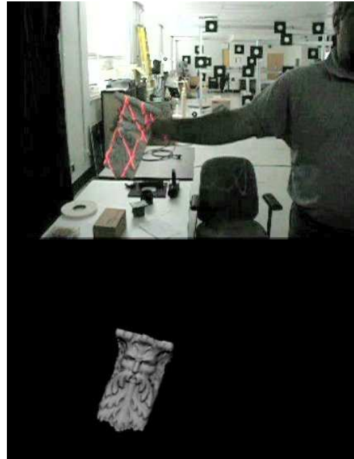
Figure 5: Hand-held 3D acquisition and real-time tracking using fast Lissajous scanning patterns. External constraints of rigidity are removed; no external positioning device is needed. This and the dual equivalent of holding the 3D camera were tested during this work. A priori object model is not needed; the model is reconstructed while tracking.
