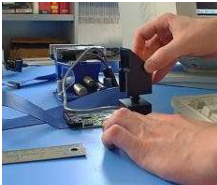
Figure 8: The optical triangulation sub-assembly, and its associated electronics.
