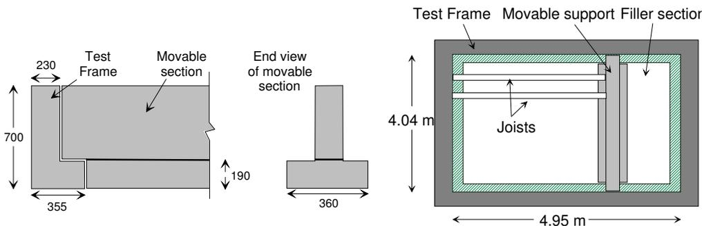
*Fig. 1: The movable support used to change the floor size by supporting different joist lengths. (dimensions in mm)*
