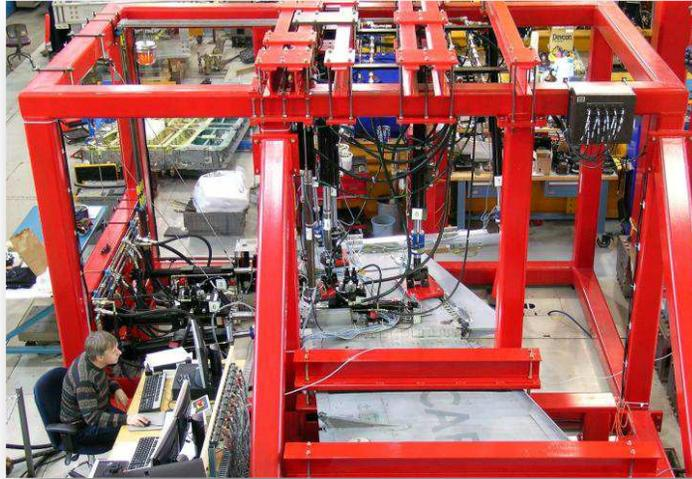
*Figure 4: CF188 outer wing spectrum loading full-scale test facility.*
