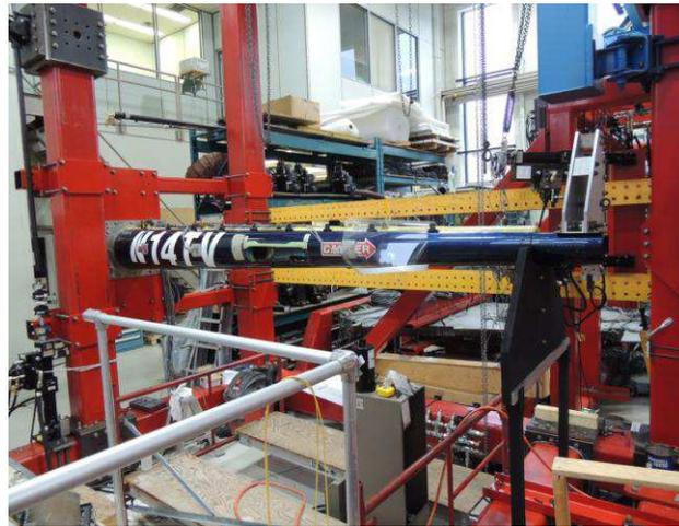
*Figure 5. Helicopter tailboom for assessing loads monitoring and damage detection / monitoring sensor performance under realistic flight loads.*
