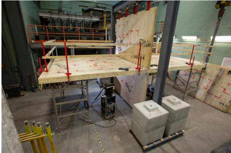
Figure 1 – Set-up for measuring the junction vibration reduction index  $k_{ij}$  at CLT floor-wall junctions
