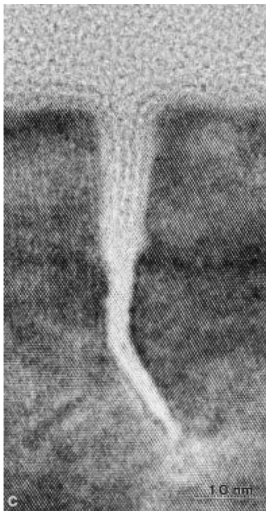
Fig. 1. Cracks in [011] cross-section of 20 nm layer sample. (a) g = 0\bar{2}2 image showing V-shaped cracks. (b) g = 200 image showing that the strain was relaxed at the tips of cracks but the areas between the crack tips are still strained. (c) HRTEM image of a crack showing that the crack deviates from the {011} plane on to the {111} plane after penetrating a distance of 10–15 nm into the substrate.
