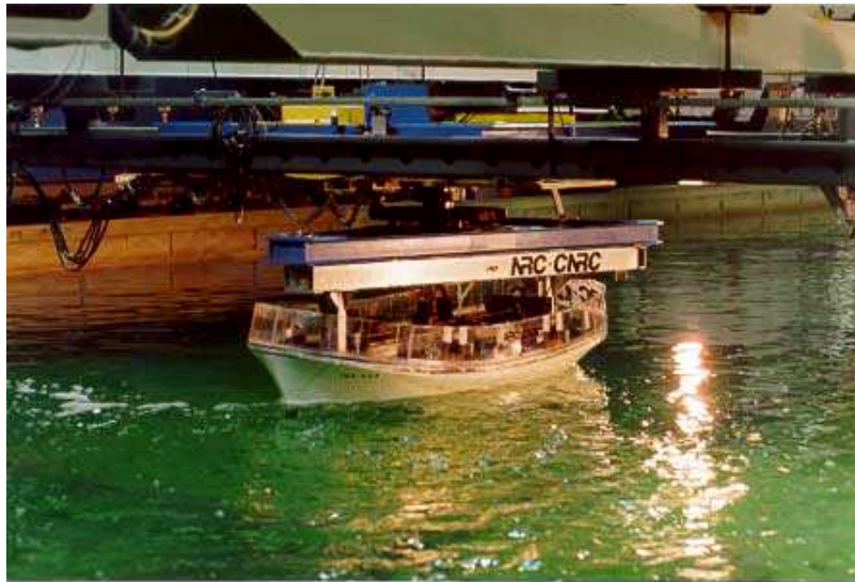
Figure 3, Tug model on planar motion mechanism
