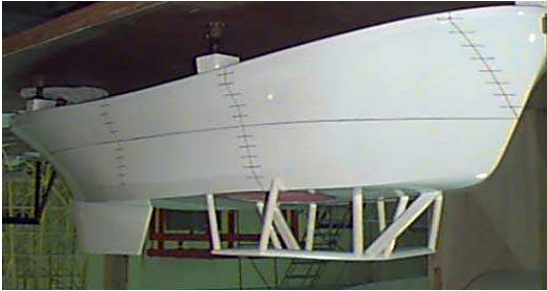
Figure 1, Tug model prior to testing, hull only.
