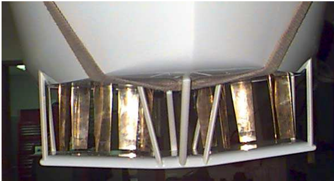
Figure 2, VSP units fitted to hull.
