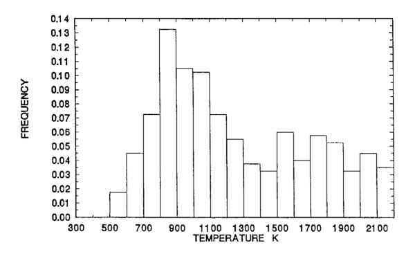
Figure 2 Temperature Histogram in Turbulent Flame Burner
