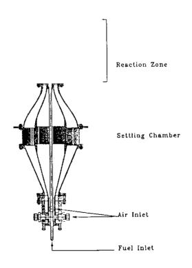
Figure 1 Schematic Diagram of Experimental Burner
