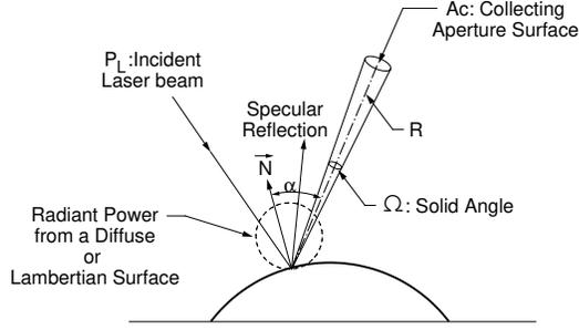
Figure 8: Effect of surface reflectivity on the received laser power.
