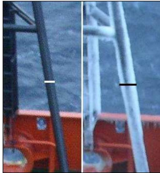
**Figure 5.** Example of an icing measurement obtained manually. The left image shows a structural component's horizontal width at the measurement location (white line) and the right image shows the width including the ice layer during an icing event (black line).
