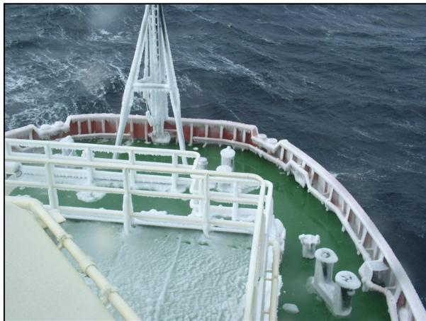
**Figure 3.** Marine icing accumulation on the deck and rail structures of the Atlantic Kingfisher.
