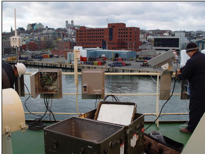
**Figure 2.** MIMS installation on the Atlantic Kingfisher at dockside in St. John's harbour. All components are attached to the railing on the top deck of the vessel. One of the camera housings is visible at the right and the power supply box and CPU box are visible at the center and left. The satellite phone antenna is visible at the far left.
