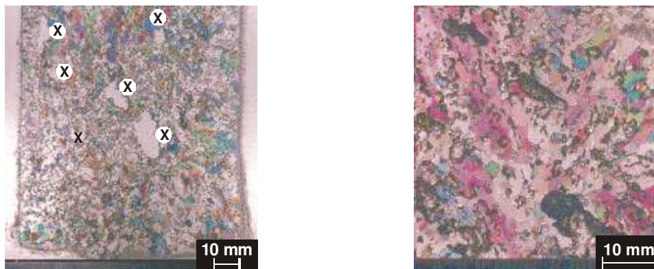
(a) horizontal thin section, with voids marked (b) vertical thin section, zoomed
