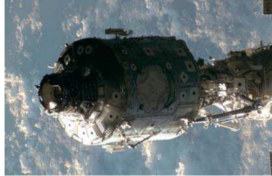
Figure 1. The existing Space Vision System (SVS) uses the known locations of the B/W targets to compute the pose of objects. Effects of sun illumination and earth albedo on video images that affect accuracy and reliability are wide dynamic range, poor signal, saturation, and shadows. (Courtesy of NASA)
