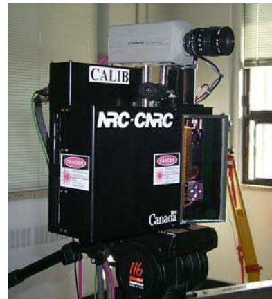
Figure 3: Prototype of the laser scanner system, a conventional video camera is “temporarily” mounted on the laser scanner for monitoring and comparison with conventional video methods.
