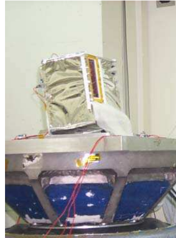
Figure 16. The Neptec Laser Camera Tracking System under vibration tests at the David Florida Laboratory. The camera head contains the entire electronics, optics, laser source, and processing computer.
