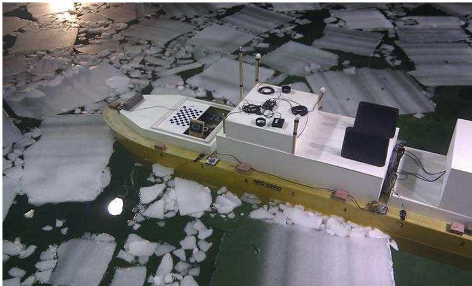
Figure 2: Model DP drillship in IOT's ice tank (August 2011).
