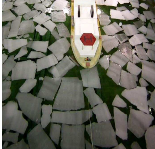
Figure 8: Numerical simulation (left) and model testing (right) after 10 seconds
