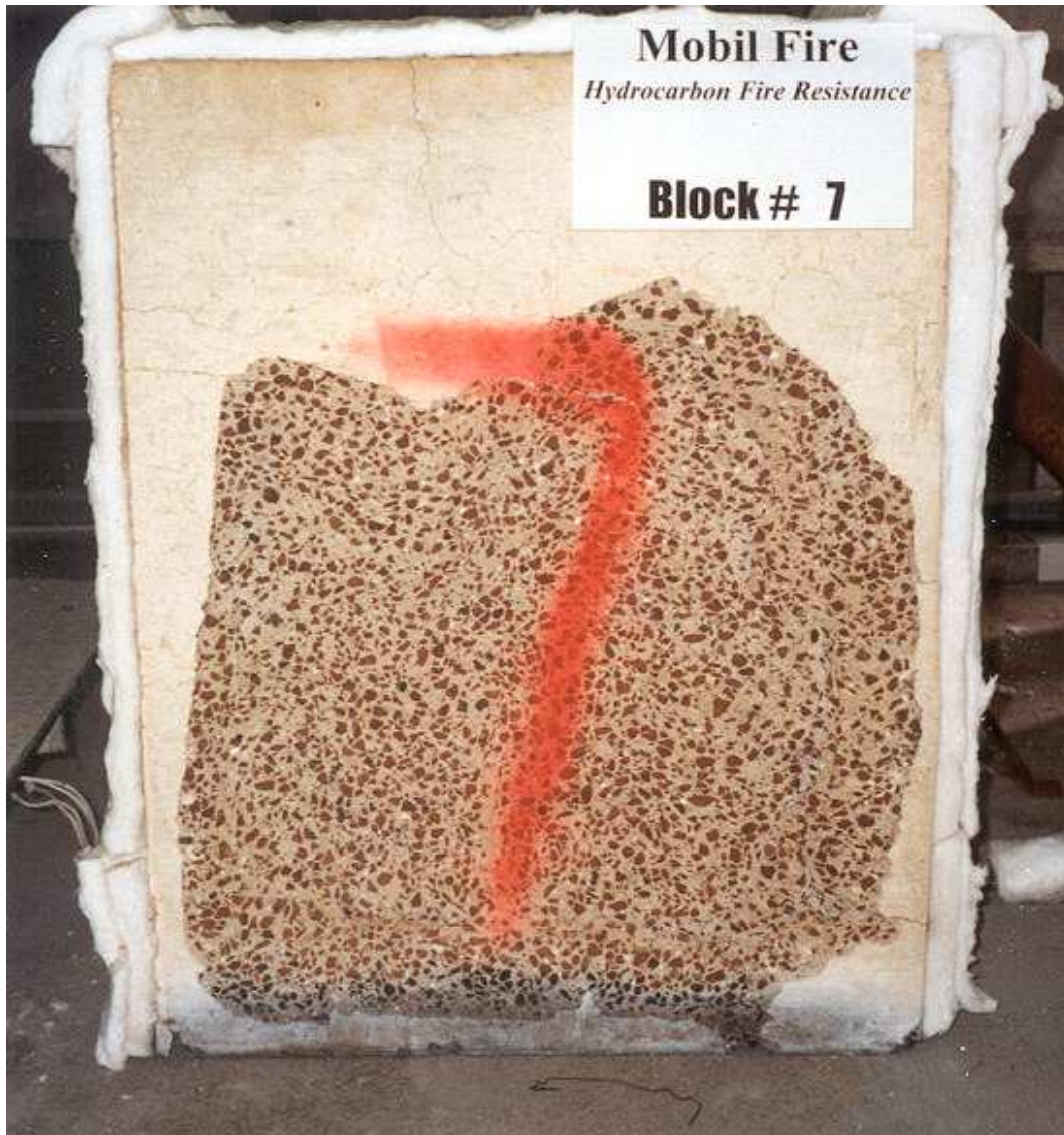
Fig. 9 – View of the Block No. 7 ( W/C = 0.33 , high-absorption coarse aggregate, 2.5 \text{ kg/m}^3 of 20-mm fibres) after the hydrocarbon-fire resistance test.
