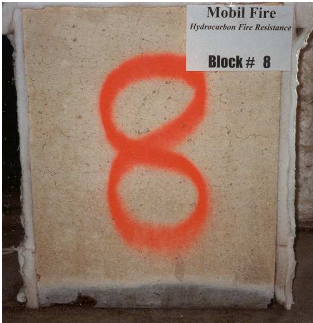
Fig. 10 – View of the Block No. 8 ( W/C = 0.33 , high-absorption coarse aggregate, 3.5 \text{ kg/m}^3 of 20-mm fibres) after the hydrocarbon-fire resistance test.
