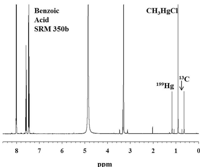
Fig. 1. Quantitative <sup>1</sup>H-NMR spectrum of CH<sub>3</sub>HgCl admixed with the NIST benzoic acid SRM 350b.
