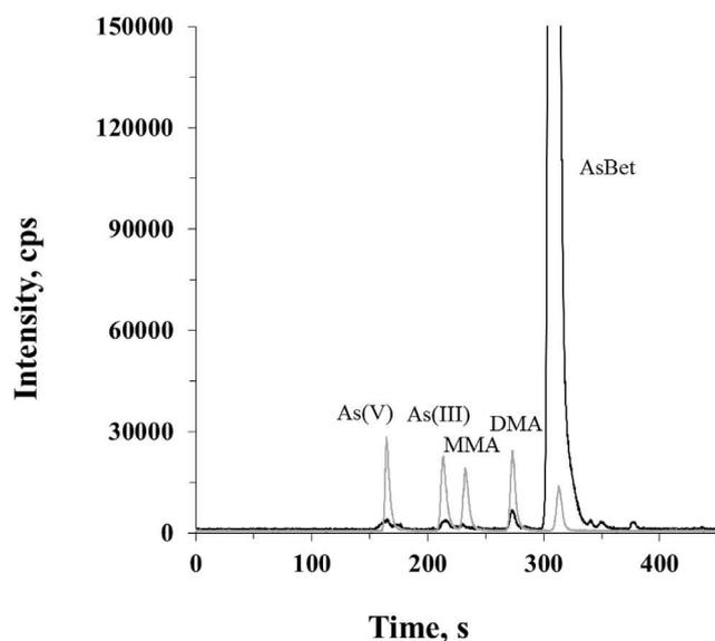
**Fig. 4.** Chromatograms obtained by LC-ICPMS from a mix arsenic standard solution of 5 ng mL<sup>-1</sup> (grey line) and SQID-1 extract (black line) on ODS column. The dead volume is at 50 s.
