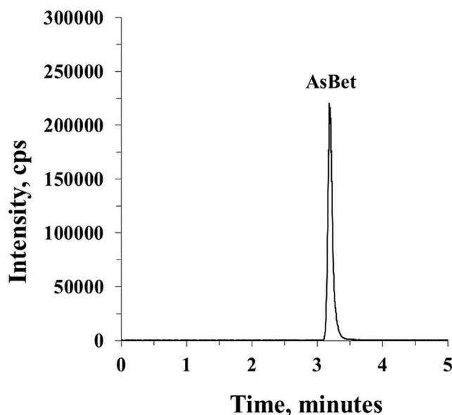
Fig. 3. Spectrum obtained by LC-MS/MS from diluted SQID-1 extract on Zorbax HILIC Plus-RR column,  $m/z$  120 from 179 monitored. The dead volume is at 1 min.
