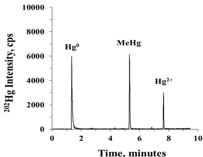
Fig. 2. A chromatogram obtained by SPME GC-ICPMS from SQID-1 extract for MeHg determination,  $^{202}\text{Hg}$  isotope monitored. The dead volume is at 0.5 min.
