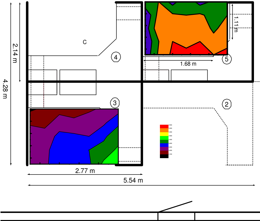
Figure 8, Contours of AI values for propagation from workstation #4 to workstations #3 and #5 from measurements at 0.30 m intervals. (Figure shows part of a 6 workstation open-plan office).
